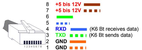
image 3: Pinout of the RJ45 connectors (IGC conform)
