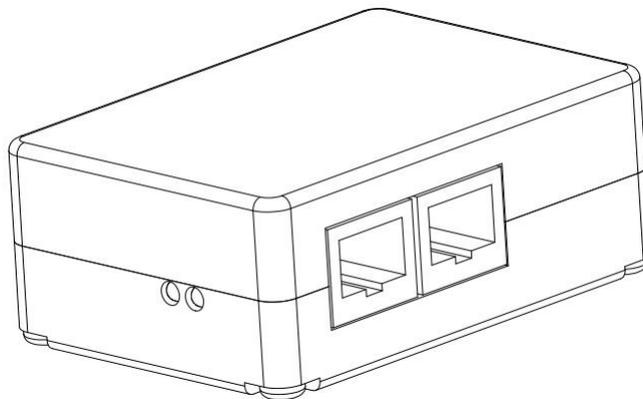
The K6 Bt provides a connection between a device with a serial RS232 port (GPS device, e.g. flight recorder, flarm, variometer) and a bluetooth enabled device (e.g. PDA, Smartphone, Tablet or PC). It is possible to send data in both directions using several baud rates. The baud rate can be configured automatically, manually by jumpers or with a compatible software. To prevent unauthorized access, the connection is password protected.
